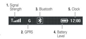
1. Signal Strength Indicator – Vertical bars show the strength of the network connection. You cannot make or receive calls when the  $\P$  (no signal) indicator or  $\P$  X (no transmit) indicator is displayed.
